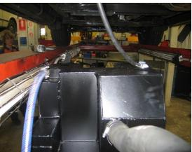
8. Prior to fitting the tank to the vehicle the fuel lines on the car need to be changed. Swap the factory hose for the supplied 8mm and 10mm fuel hose. Furthermore, on the rear right hand mounting bracket, the locating dowel on the mount needs to be removed. Using vice grips locked on tight to the dowel, simply bend backwards and forwards to break the dowel off.
