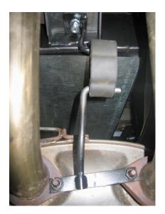
13 Connect up the filler pipe with the supplied hose, along with the breather line to the standard filler. (Note: image is shown of an FG utility).
