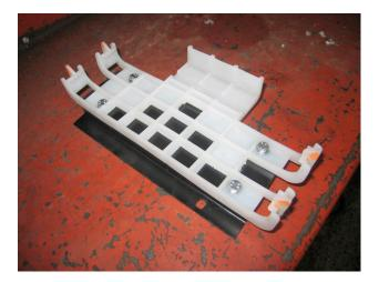
Fit the carbon canister/bracket to the front left of the tub wall, by drilling through the tube, and fastening with supplied bolts.
