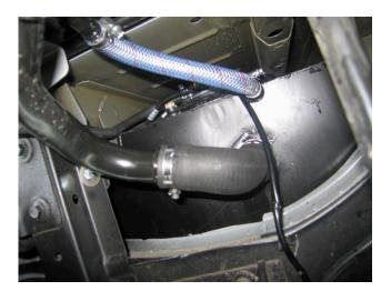
14 Check all tank fittings and hoses are tight, before filling tank with fuel. Test drive the vehicle to check for any possible leaks.
