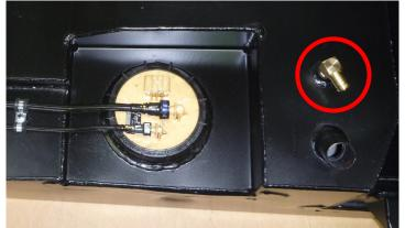
10. Fit filler and fast fill hoses to the new tank. Take note of the position of the hoses before removing them from the standard tank. Fit hoses to the new tank in the same position as they were removed from the standard tank.
