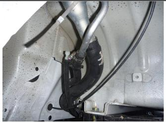
2. Lift car on hoist or jack stands to remove the fuel tank. Unclip fuel lines from front of tank making sure lines don't syphon fuel onto the ground.
