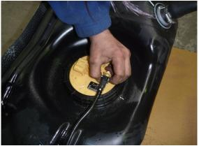
5. Remove fuel sender unit. This requires a special tool. In the absence of the special tool, the sender outer ring can be undone using a hammer and a blunt piece of metal. Tap lightly on alternating sides of the ring changing ribs regularly to avoid breaking ribs
