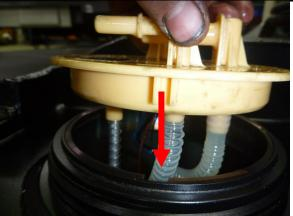
7. Fit the fuel lines to the new tank. Fit the cushion clamps to hold lines in place and then tighten using M6 nuts and washers supplied.
