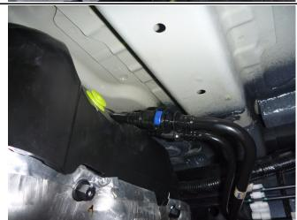
3. Undo front and rear mounting straps from under the tank, keeping bolts to be used on the new tank. Lower tank down carefully to gain access to fuel pump/sender unit wiring, unclip plug from gauge, then lower the tank to the ground.
