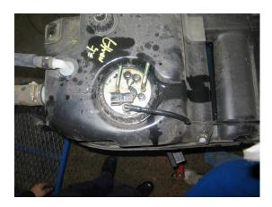
6. With the sender unit out, take a small flat head screw driver to lever off the pick up filter from the bottom of the unit being careful not to damage the retaining clips. Once removed, the very base of the pick up needs to be cut at 45 degree's to the bottom of the pickup as shown. After trimming, file the edges smooth and thoroughly blow out the pick up to ensure no filings remain in the pick up before re-installing the filter to the bottom.
