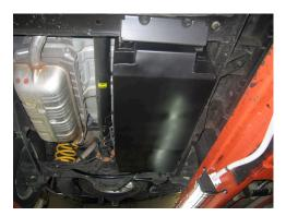
10. Re-connect the fuel filler hose and TMP breather hose to the filler tubes. For the 6mm fuel hose breather line from the discriminator valve, route this along the top of the filler tubes up into the wheel arch near the fuel door. Retain with zip ties, and fit the supplied fuel filter to the top of this hose as shown.
