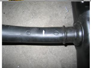
10. Drill 12mm hole in the top of the filler and fit the 5/8" x 1/4" fast fill breather and seal with araldite.
