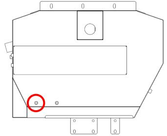
Using Teflon tape, thread sealant or the likes, install BRASS – ELBOW - 5/16" x 1/4" BSP to the circled socket.
