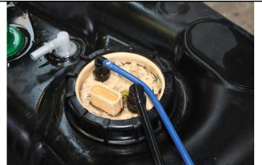
6. Remove fuel sender unit. This requires a special tool. In the absence of the special tool, the sender outer ring can be undone using a hammer and a blunt piece of metal. Tap lightly on alternating sides of the ring changing ribs regularly to avoid breaking ribs.
