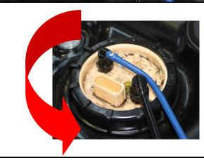
7. Fit gauge into Brown Davis tank with original gauge ring and seal. Fit 8mm fuel hoses supplied in kit.
