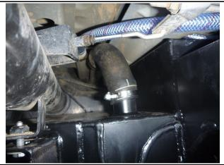
15. Fit SET SCREW - HEX - M10 x 100mm, through the original hole in the front cross member. You may have to drill through the top of the cross member for the bolt to go through.
