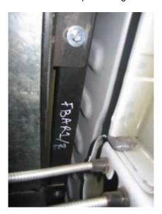
11 Re-connect the fuel lines to the factory fittings, and where possibly, using the factory fuel line fittings.
