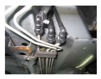
Resecure hand brake cables by modifying the standard mount with the exhaust. See image below for directions.
