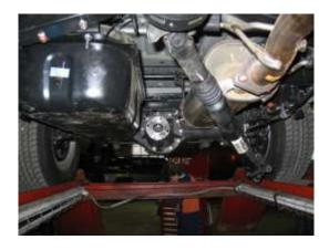
2. Undo the factory fuel breather line from the passenger side outer chassis rail.
