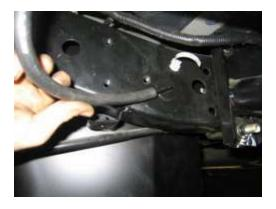
13. The fuel delivery and return hoses now need to be trimmed to suit and fitted to the factory fuel lines. Be sure to get the right hoses on the right position, these should have been marked earlier when they where undone.
