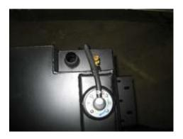
8. Prior to lifting the tank into position, in order to make the installation easier, clip the fuel gauge sender unit extension loom onto the tank gauge sender unit boss now. As there is little room for hand access once the tank is lifted into position this will make the connection easier when lifting the tank into position.
