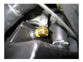
12. Connect up the breather line running to the factory breather connection on the passenger chassis rail. Trim hose if required.
