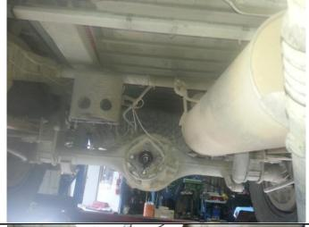
2. Remove exhaust. The exhaust unbolts at the same point as the tail shaft.
