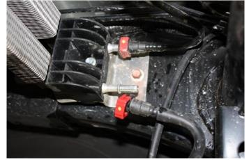
4. Lower the tank down further, removing the sender plug wire, leaving the fuel lines on the tank, then lower the tank all the way out of the vehicle.
