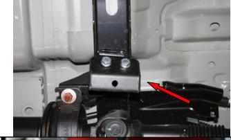
9. Use a lifting device to raise the new tank into place.(Whilst lifting the tank, fit the sender wire as shown).
