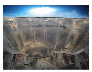
With the standard tank removed, begin transferring the fuel gauge sender unit into the new tank. When installing the sender, sit the unit alongside the tank at the height where it will be located when installed in the tank, and check the travel of the float arm to ensure that it will read accurately. It is more important to ensure that empty is accurately read rather than indicating full. The sender float arm can be bent by hand to obtain the correct travel arc.
