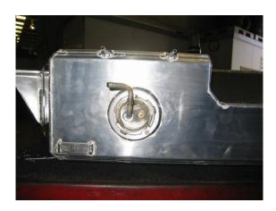
3. With the supplied filler hose, remove the filler nozzle from the standard tank filler tube, and fit to the new tank.
