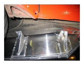
6. Complete the installation by re-connecting the fuel pick up and breather lines to the new tank. Add fuel to the tank, and check fuel gauge function progressively when filling. Inspect thoroughly for any potential leaks or areas of hose/wire that may be in contact with the tank that might cause damage over time.
