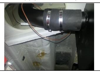
24. Double check all fuel line clamps and security of fuel lines. Fill tank and check for leaks. Road test and check for rattlers & squeaks. Re-check for fuel leaks.
