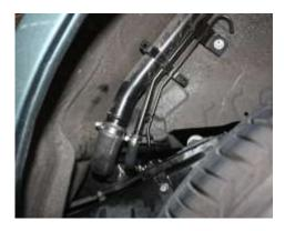
13. Fit fuel lines to sender with supplied hose clamps. Make sure fuel line is clear of tank and not jammed.
