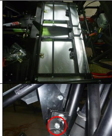
22. Drill a hole to fit an M10 bolt through in the side brackets of the seat frame.
