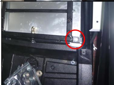
23. Fit a M10 bolt with washers and nut into the brackets at the front of the frame
