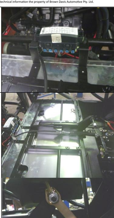
25. Reinstall the gear shifting mechanism
