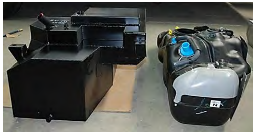
Brown Davis replacement tank next to vehicle's standard tank
