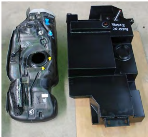
Brown Davis replacement tank next to vehicle's standard tank
