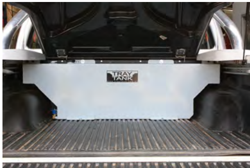
Fuel Tray Tank fitted in Dual Cab ute
