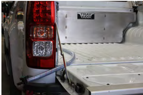
Water Tray Tank fitted in Dual Cab ute Gravity feed tap system shown
