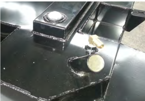
Filler point / Fast fill breather / Roll Over Valve
