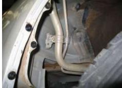
6 With the guard liner removed, using a 12mm socket/spanner undo the filler neck mount bracket bolt. Furthermore, underneath the car there is another mount bolt that needs to be undone to allow removal of the entire filler tube.
