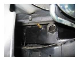
23. The filler tube supplied can now be joined using the hose and hose clamps supplied. Note the orientation of the filler tube in the images below. Once in place and fastened, proceed to check all connections and hose clamps on the dual filler neck to ensure proper fitment.
