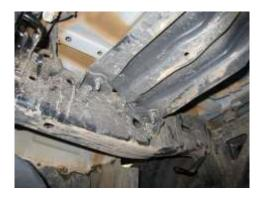
3. Proceed to undo the two brackets left on each chassis rail. Remove all 6 bolts using a 12mm socket/spanner.
