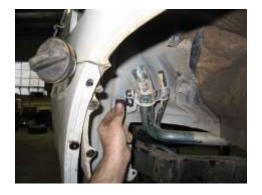
The supplied dual filler neck can now be installed. As indicated in the pictures below, the circular cutout in the filler neck needs to be pointing towards the ground to be at the correct orientation (angle can be adjusted slightly to suit). Once in place, join the filler neck to the factory filler tube as shown with the supplied rubber joiner and hose clamps.
