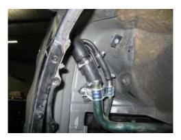
11. The fuel filler line for the transfer pump now needs to be fitted to the second (lower and rear pointing) outlet on the new filler neck. Fix in place with the hose clamp provided, and route the hose along the filler tube down to under the vehicle as shown.
