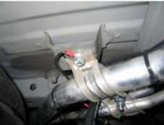
14. The second of the wires can be left at full length and routed to where the centre of the tank will be when in position (will be trimmed when the tank is being fitted).
