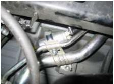
13. Wiring for the transfer pump and gauge now needs to be run from the engine bay. Route some dual wire down the driver's side of the car. One of the wires needs to run power to the transfer pump, and the other wire will be used as the signal wire for the fuel gauge sender unit.
