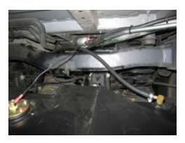
17. The front tank brackets also need to be drilled through the chassis cross member. With the tank pushed up and the side rear brackets in place beneath the tank mounts, take a drill with 10mm drill bit and through the cross member using the already drilled tank bracket as a guide.
