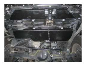
25. Using a 12mm socket or spanner, all tank mount bolts can now be tightened firmly. Once all bolts are tightened, proceed to double up the M10 nuts on each bracket mount with the nuts provided to ensure a very rigid mount. With all bolts now fastened, trim the excess wire from the mount bolts where they entered through the chassis rail/cross member openings using side cutters.
