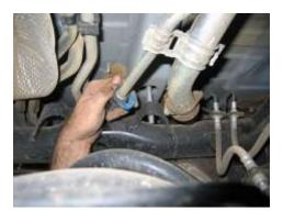
5 The inner guard lining drivers side rear wheel arch needs to be removed to gain access to the filler neck. Using an allen key, undo and remove the liner, retaining the screws.
