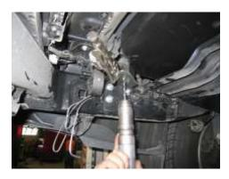
21. The transfer pump fuel hose routing now needs to be completed. With the hose routed earlier from the tank pick up over the diff/chassis cross member, trim the hose to length to allow fitment of the supplied fuel filter between the pump and the tank as shown and fasten with hose clamps supplied.
