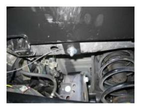
18. The spare wheel frame is to be re-installed next. However a minor modification now needs to be made to the centre of the mount as shown. With a hacksaw, make cuts approximately 25mm apart as shown and fold this over with a hammer. This will allow clearance in order to bolt the frame brackets back in.
