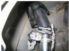
10 Proceed to fit the filler neck breather line with the hose and clamps provided between the factory filler tube breather and the new filler neck as pictured.
