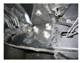
20. The tank should now be in place with bolts only finger tight. Using vice grips or similar clamping tool, clamp the rear tank brackets to the rear tank mounts in order to be able to drill both brackets for mounting. Once clamped, pilot drill holes using a 5mm drill bit, before drilling with a 12mm drill bit to finish off. Fit two M10 screws, M10 flat washers, M10 star washers and M10 nuts through the brackets and tighten firmly.
