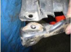
19. With the tank now resting on the spare wheel cross member, fit the left and right rear mounting brackets as shown.
