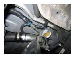
22. The tank filler neck and breather lines now need to be attached to the fuel filler. Starting with the straight brass fitting supplied, coat the thread with pipe thread sealant and fit into position. Proceed to route a piece of supplied fuel hose between this brass fitting and the rear most vacant breather outlet on the dual filler neck and fasten with hose clamps supplied.
