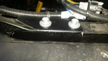
8. Fit the MOUNTING BRACKET WITH 4x M10 CAPTIVES (TB-TL79R4-3) to the four original tank support rail captives
