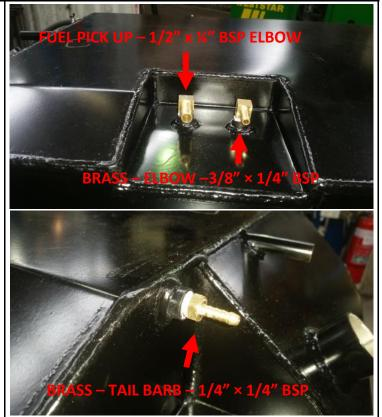
10. Remove the check valve line off the standard tank and connect it to the BRASS - TAIL BARB - 1/4" x 1/4" BSP fitted in previous step.
