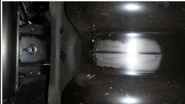
4. Carefully lower the tank out of the vehicle.
