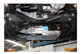
4. Fit the guard with the supplied M10 fasteners. The front 3 and rear 2 bolt holes require M10 x 25mm screws. The middle 2 bolt holes require M10 x 75mm bolts which screw into the supplied back up plates.
