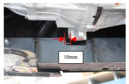
3. Fit the brackets with the factory bolts
