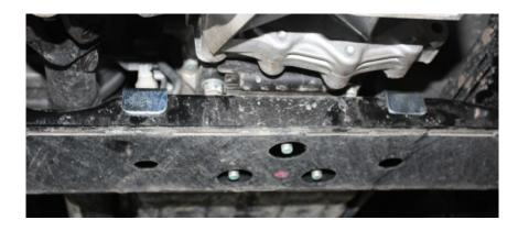
3. Slide (UGNND40T2) under the front guard (UGNND40F1)
