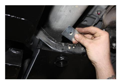
4. Slide (UGNND40T2) under the front guard (UGNND40F1)
