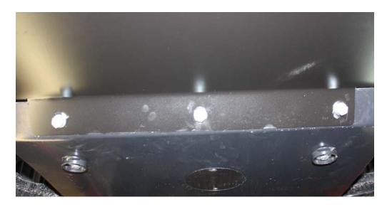
4. Refit gearbox cross-member supports using standard bolts (as shown below)
