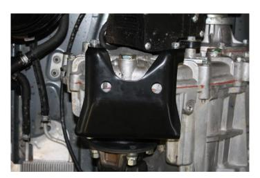
2. Fit the 2x guard brackets to the transfer case using standard bolts (as shown blow) and tighten.
