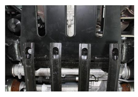
2. Fit M8 saddle captive (BP-CF-8-050092) over existing hole on standard sump guard aligning it with the hole
