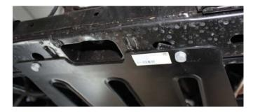
2. Remove 4 M8 bolts from rear of the front standard sump guard
